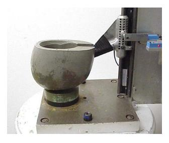
SwRI Helmet Test Equipment Photo 2. Flat Anvil Impact Configuration
