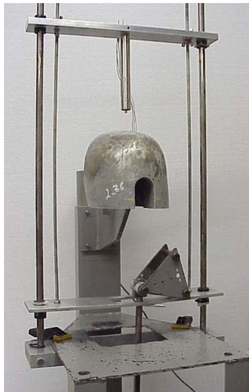
**SwRI Helmet Test Equipment Photo 6. Retention System Tester with Supported DOT Headform,
