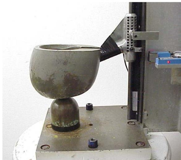
**SwRI Helmet Test Equipment Photo 3. Hemispherical Anvil Impact Configuration**
